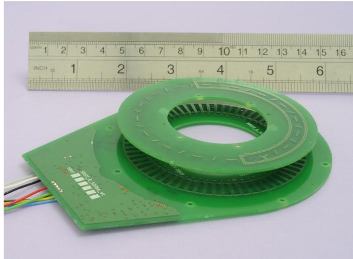
Fig. 3 – An example of a bearingless Zettlex rotary encoder – ideally suited to harsh environments.
